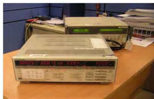
Fig. 2 AC power Calibrations System for Digital Wattmeter
